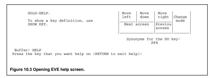
As the bottom of the screen tells you, you can display help about a specific key by pressing that key while viewing this screen. For example, press F1 (the Find key—as the diagram shows, this is the upper-left corner of the numeric keypad, which is NumLock on a PC and PF1 on an actual VT terminal) to display help about searching for text, as shown in Figure 10.4.
