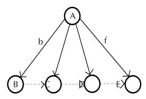
The graph of an object's instance is dynamic, representing its state at a given time. For example, this graph shows a QStack object that currently has four items. Solid arrows show the composed-of edges and dotted arrows show ordering edges. The b and f on the graph show that two composed-of edges of the QStack are used as pointers to the back and front of the stack.
